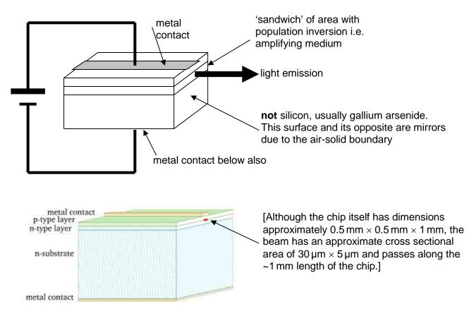
The above laser fits the basic shape of a normal laser (shown below).
