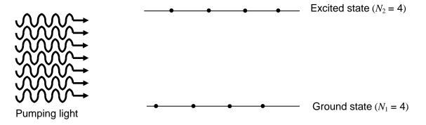
In this situation the incoming flood of photons is just as likely to cause an electron to drop (stimulated emission) as it is to cause an electron to rise (absorption). The best we can achieve here is  $N_2 = N_1$  which is not quite good enough.
