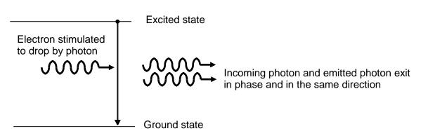
The reason that the electron is stimulated to drop is that the incoming photon is an electromagnetic wave and its e-m field will exert an oscillating force on the excited electron. If the incoming photon is of the correct frequency, this oscillating force will cause the excited electron to drop and both photons will exit with the same frequency, phase and direction. Note: again, the incoming photon needs to be of the **correct** energy.
