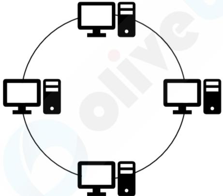
In ring Topology, network nodes are connected in a closed loop configuration. Each node has directly connected with its adjacent node on both sides. The Others are indirectly connected and the data passing through one or more intermediate nodes.
