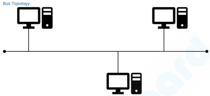
In the Bus topology system, every computer and network are connected by using a single cable. The cable is known as Bus. It transmits the data from one end to another end only in a single direction. When it has exactly two endpoints, then it is called Linear Bus topology. A network that uses a bus topology is referred to as a bus network. Bus networks were the original form of an Ethernet network.
