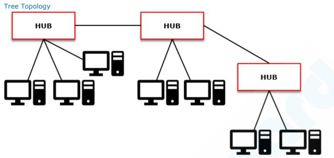
In Tree Topology network, two or more-star networks connected with a root node and all other nodes are connected to it forming a hierarchy. It is also called hierarchical topology. It should at least have three levels to the hierarchy. This type of topology used in Wide Area Network. Tree topology is valued for its scalability and accessibility for troubleshooting.
