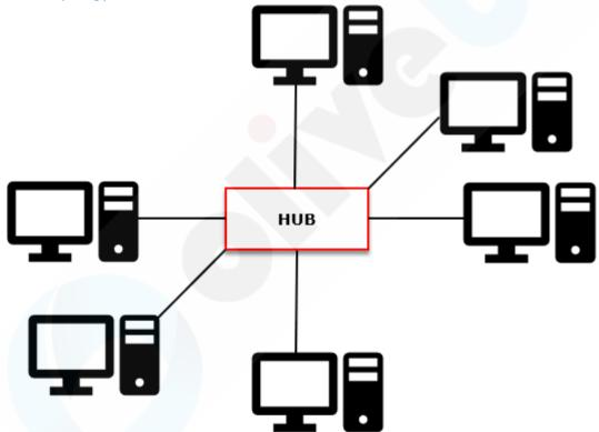
In a star topology, all the nodes are connected to a single hub through a cable. This hub is the central node. The data can send from one node to another through the hub. Hub acts as a repeater for data flow. It can be used with twisted pair, Optical Fibre or coaxial cable.
